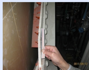
Center plate with a few millimeter bent
